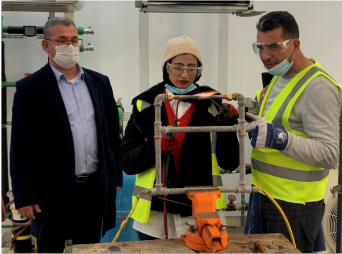
Brazing under nitrogen flow
