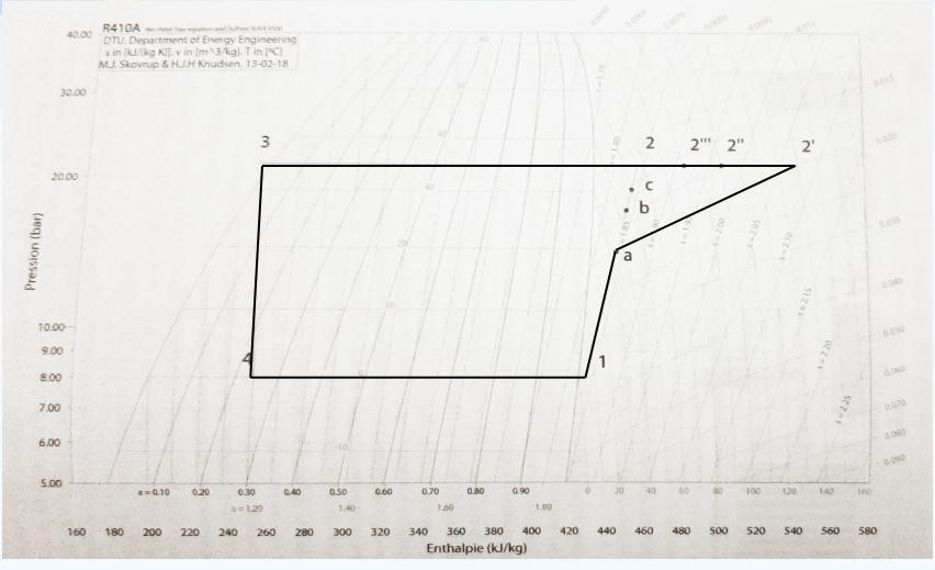
Plotting refrigeration cycles on the enthalpy diagram
