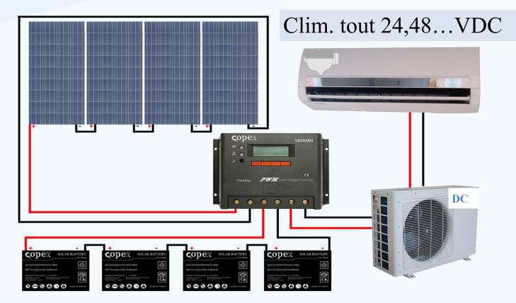
100% DC system, the regulator is used to guarantee a constant DC voltage to power the air conditioner
