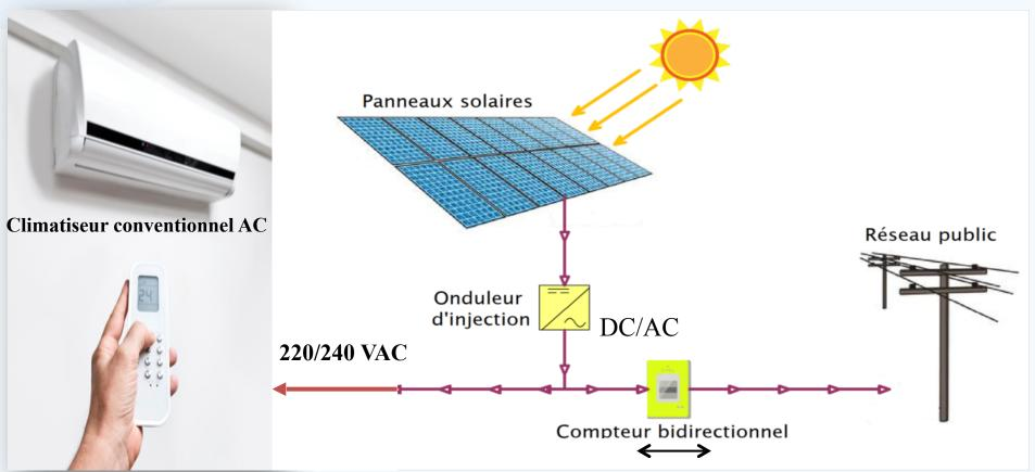
A supply voltage is always guaranteed by the electricity distributor. The PV field is used to  $_{14}$  educe the consumption bill by counting the injected KWh.
