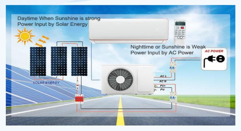
The system operates mainly by solar energy, when the light is not sufficient, standard electrical energy comes in as a backup, the adaptation of this energy mix is done automatically according to the cases
