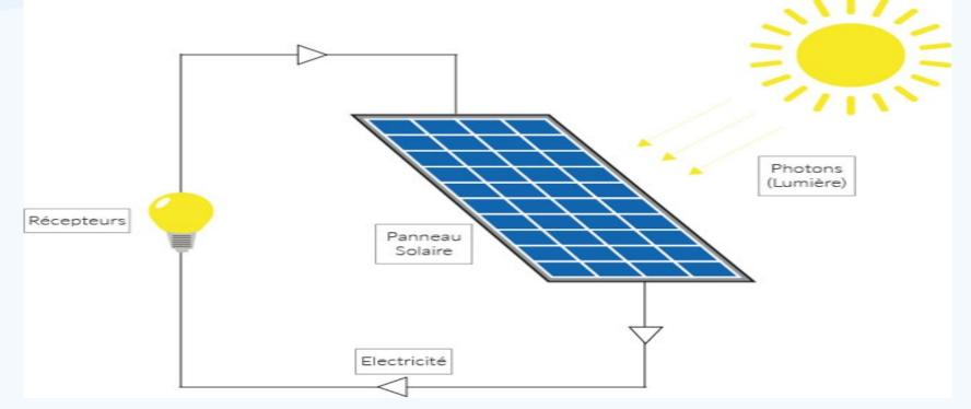
The photovoltaic cells that make up a PV panel exploit the photoelectric effect to produce direct current "DC" by absorbing solar radiation.
