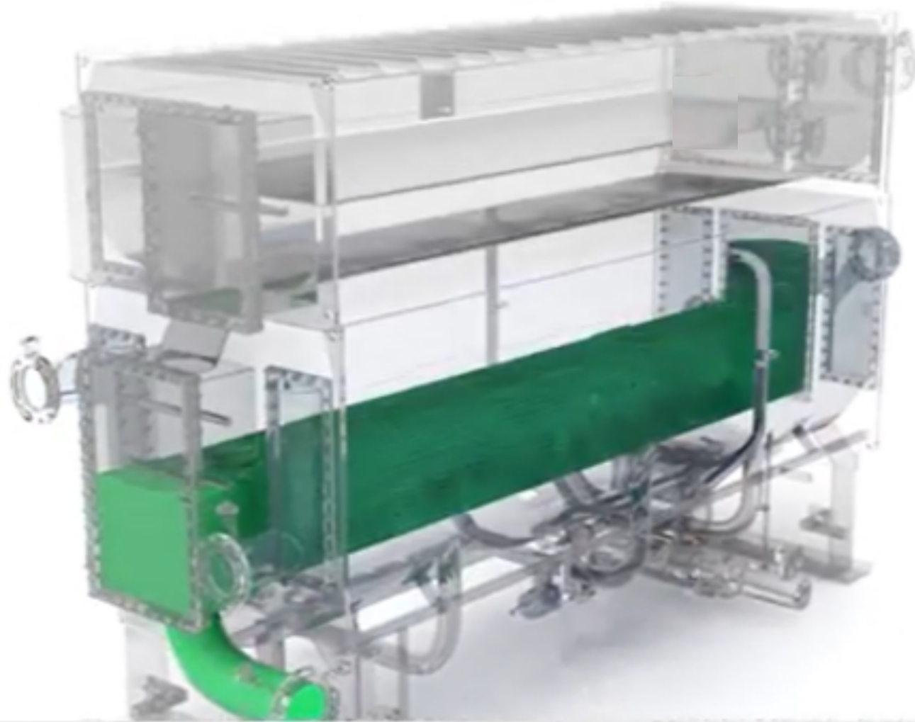
Heat of Dilution is rejected to the cooling tower water circulated inside the absorber tubes
